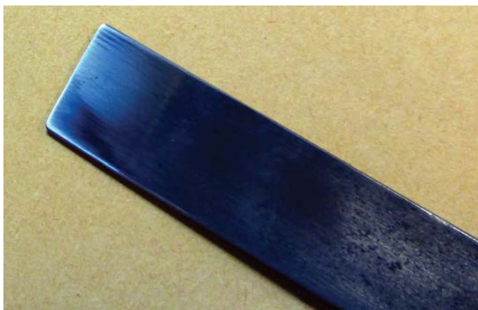
A No. 3 gouge with the corners nicely squared. A minute amount of rounding is better than the corner coming to a point
