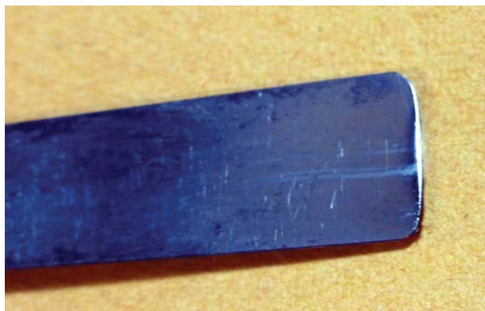
A badly sharpened gouge with the corners rounded, which limits the use of the tool
