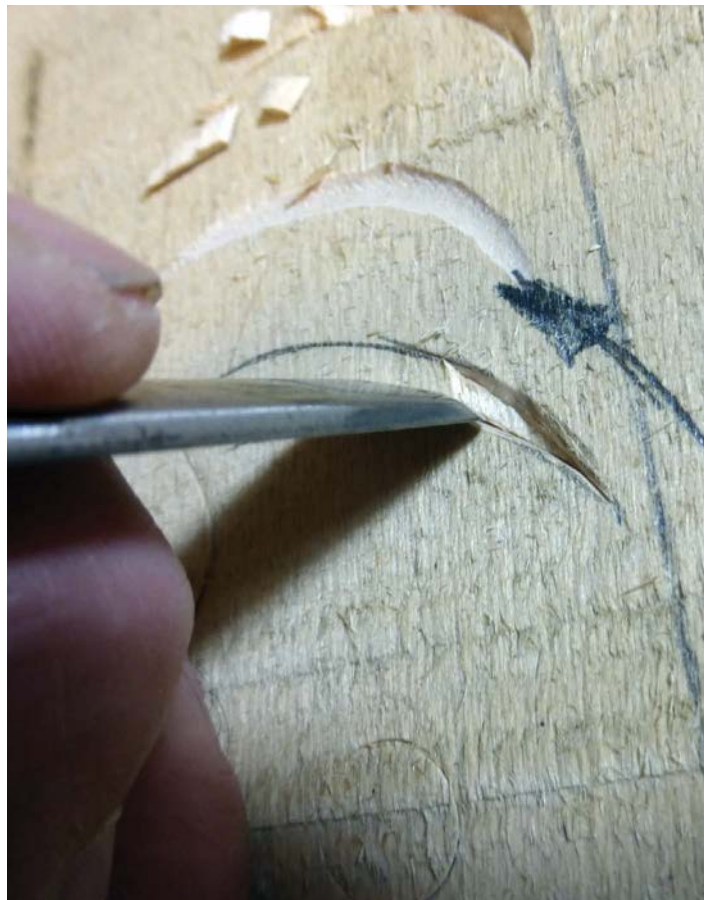
Practising the use of the bull nosed No.3 gouge on a piece of waste with a slicing motion side to side
