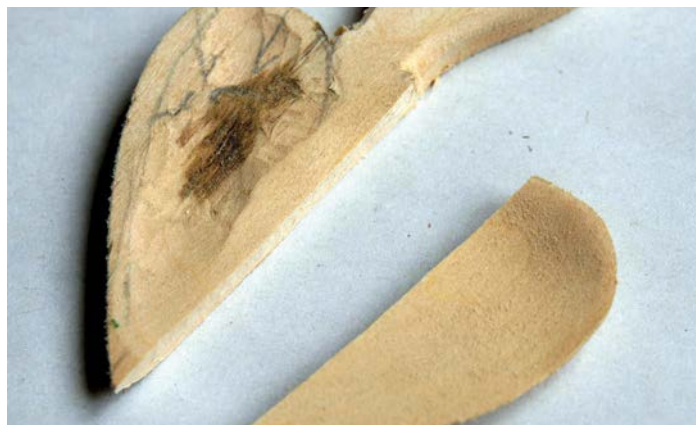
1. A clean break can generally be glued back in place, leaving little evidence of the damage.
