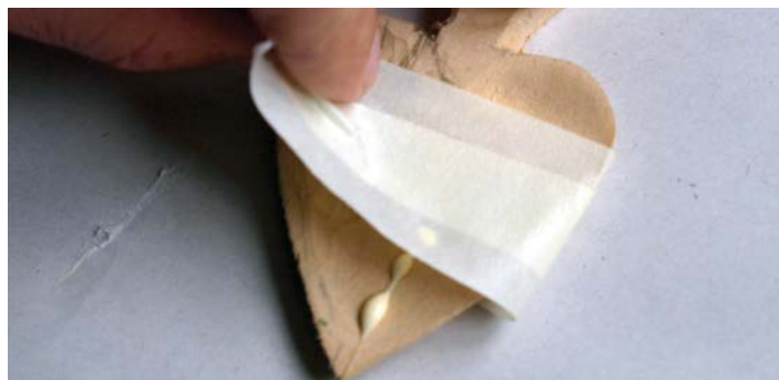
4. Sometimes it is difficult to use clamps to bind a break. Try a doubled up strip of masking tape to make a versatile and contour fitting clamp. It is possible to exert great clamping force with double layer masking tape, so avoid pulling too hard.
