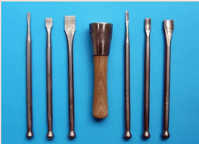
Stone carving tools: Mason's dummy mallet with three chisels and three gouges in sizes 6mm, 13mm and 18mm
