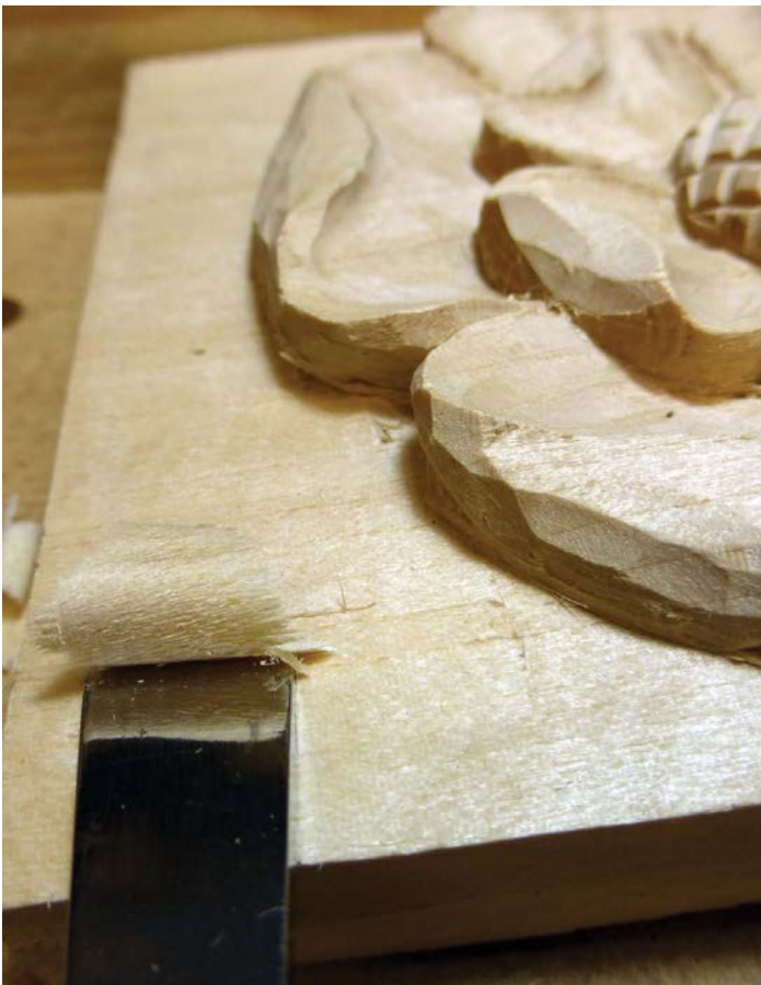
Trying to use a No.1 flat chisel to remove waste. Note the damage at each end of the cutting edge
