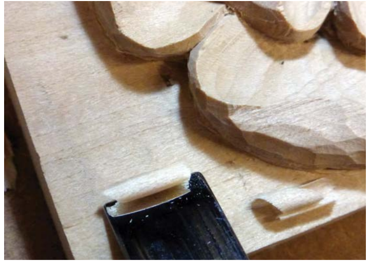
Using a No.3 gouge for removing waste on a relief carving. Note that the tool is not cutting at each end of the cutting edge, thus leaving no damage to the surface
